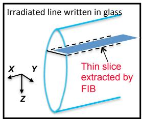
Laser-induced phase separation  $\text{Li}_2\text{O-Nb}_2\text{O}_5\text{-SiO}_2$   $\rightarrow$  LiNbO<sub>3</sub>(crystal)+SiO<sub>2</sub>(glass)
