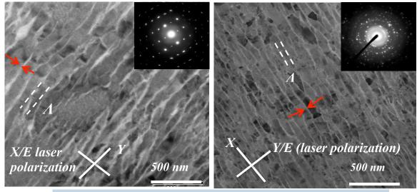
Orientable nano-crystallization and nano-structuration in glass
